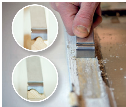
A small scraper is easy to use to sand and shape edges.
