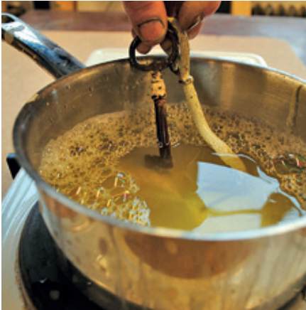
Clean fittings of paint and rust by boiling them in Linseed soap.
